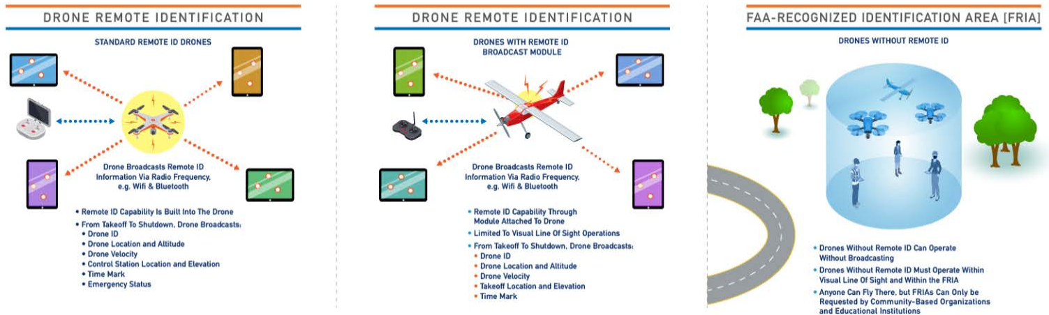
Figure 2 – Overview of Methods of Compliance in the Final Remote ID Rule, Source FAA
